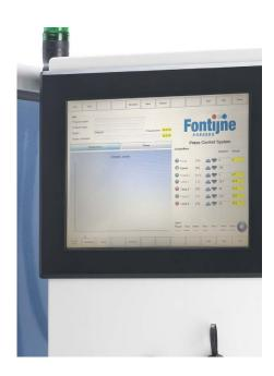
Lab technicians can easily build and store up to 999 press recipes, using the built-in preset builder. Starting a preset will fire up the corresponding process cycle automatically and will execute all programs commands and events.
